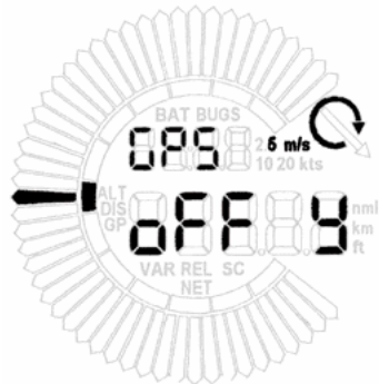
Fig. 13 GPS input not active GPS data present
