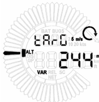
Fig 10 Landing place elevation input (target)
